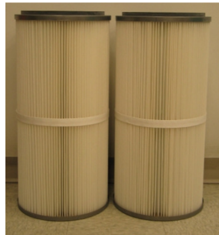
Sample 2. Arioso M7001-11 Cartridge Pair 142 Pleats, 98 ft 2 (9.1 m 2 ) of media.
